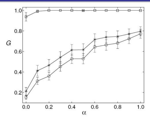
Fig. 2. Cascading failure in scale-free networks with scaling exponent  $\gamma=3$ , as triggered by the removal of one node chosen at random (squares), or among those with largest connectivities (stars) or highest loads (circles). Each curve corresponds to the average over 5 triggers and 10 realizations of the network. The error bars represent the standard deviation. The number of nodes in the largest component is  $5000 \le N \le 5100$ .
