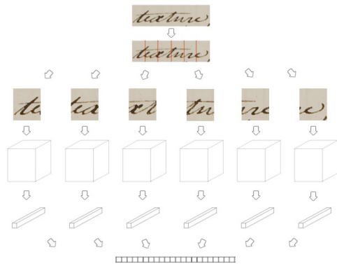
Figure 1. Processing pipeline to construct ZAH features. From top to bottom, we have: Input word image ; partition of image along its width into Z = 6 zones, with each zone covering an area of h \times w_z pixels; extraction of pixel-level hypercolumns, for each zone a h \times w_z \times d , where d is hypercolumn dimensionality; aggregation of hypercolumns into a single 1 \times d hypercolumn per zone; concatenation of zone hypercolumns into a single 1 \times Zd vector.
