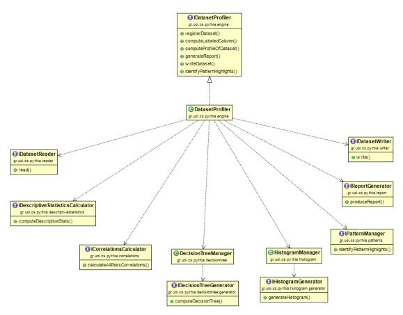
Figure 4. UML diagram with the main interfaces of Pythia.
