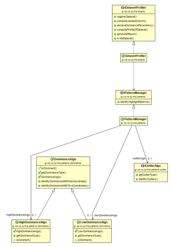
Figure 7. UML diagram with the interfaces and abstract classes within the patterns package.
