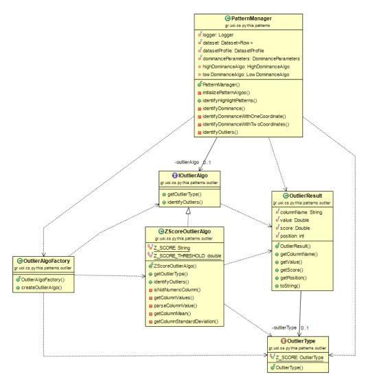
Figure 13. UML diagram with the classes of the outlier sub-package.
