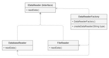
Figure 2. UML diagram with a demonstrative implementation of a parameterized Factory pattern in combination with an interface where expected behavior is defined
