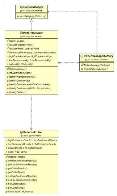
Figure 8. UML diagram with the classes directly under the patterns package.
