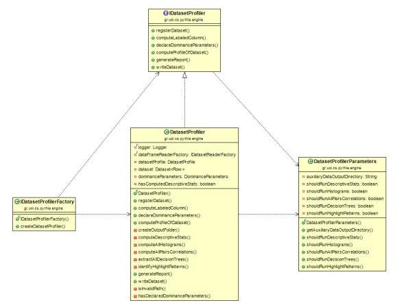
Figure 5. UML diagram with the classes of the engine package.
