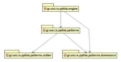
Figure 6. UML diagram with the sub-packages in the patterns package.
