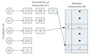
Figure 2: A simple inverted file index scheme for the example of Figure 1.
