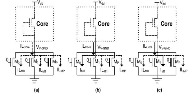
Fig. 2. Proposed scheme: (a) Snore Mode, (b) Dream Mode, (c) Sleep Mode
