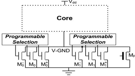
Fig. 3. Reconfigurable architecture
