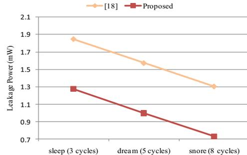
Fig. 4. Leakage power comparison between [18] and proposed architecture
