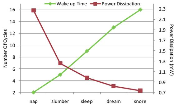
Fig. 7. Tradeoff between wake-up time and power consumption with 5 modes
