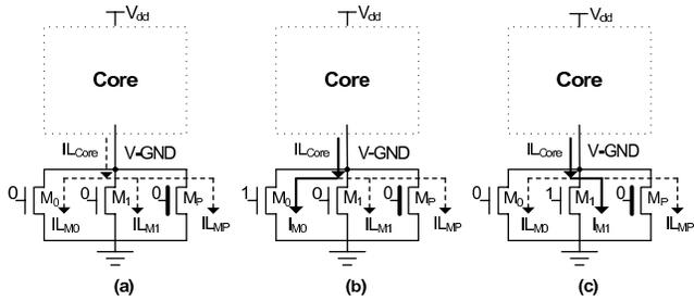
Fig. 1. Power-switch architecture [12].
