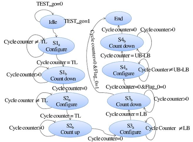
Fig. 4. Finite-state machine for BIST scheme.
