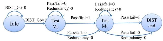
Fig. 6. BIST and Repair State Diagram
