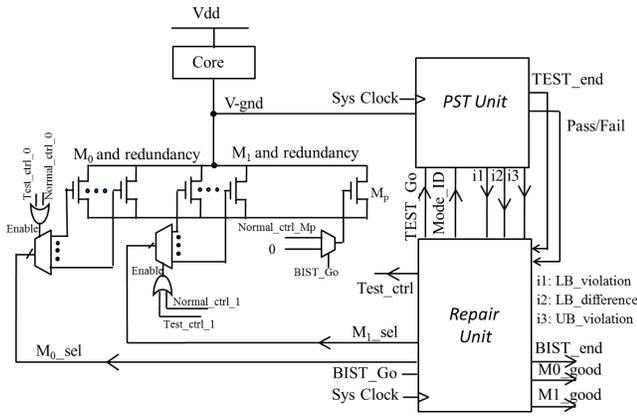
Fig. 5. The complete BIST scheme with built-in self-repair.
