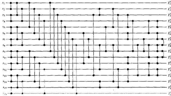
Figure 2. Optimal 16-input SN from [19].
