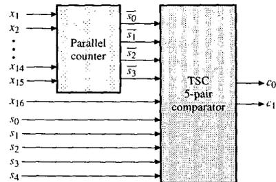
Figure 5. Internal structure of the PC-based STC for the modified Berger code  $C_{(16,5)}$ .
