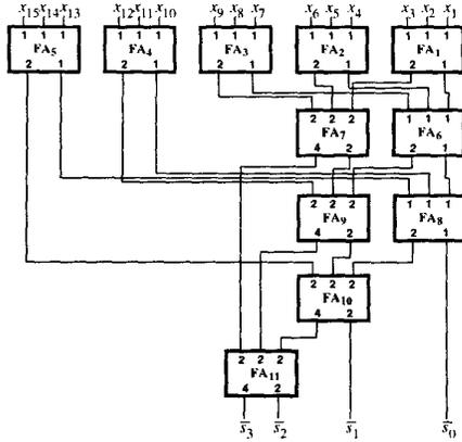
Figure 6. 15-input parallel counter.
