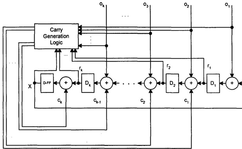
Figure 5: The proposed scheme behaving as a Multiple Input Non-Linear Feedback Shift Register
