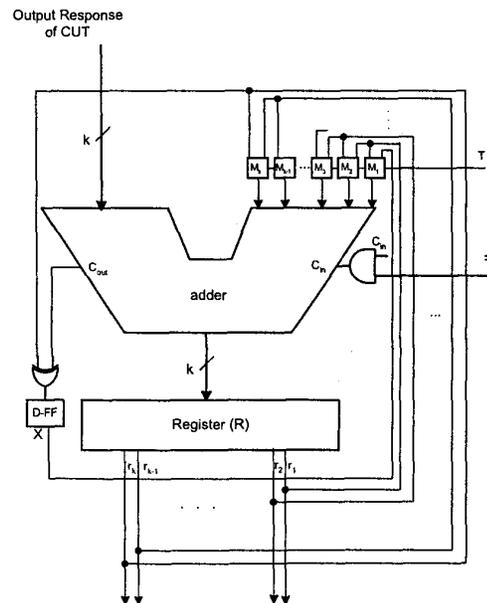
Figure 4: The proposed scheme for response compaction
