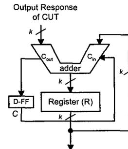
Figure 2: RCA for response compaction
