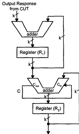
Figure 3: CC for response compaction
