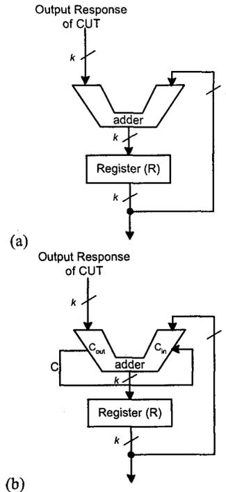
Figure 1: ABC for response compaction: (a) with 2's complement adder, (b) with 1's complement adder
