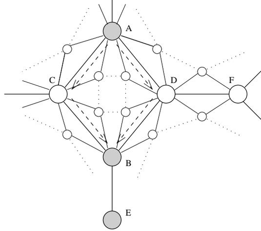
**Fig. 3.** A big  $a$ -split from  $A$  to  $B$ . Flag nodes are not shown, the shaded nodes are already explored.
