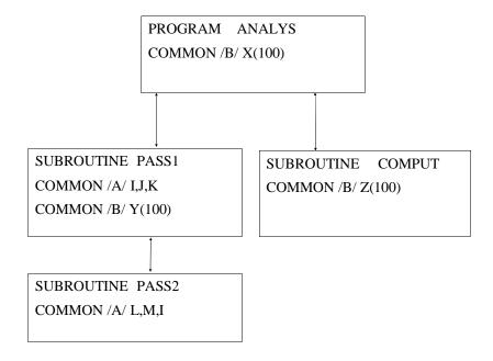
Program ANALYS has 'calls' to the subroutines PASS1 and COMPUT, and PASS1 has a 'call' to subroutine PASS2. This is summarised diagrammatically below:—
