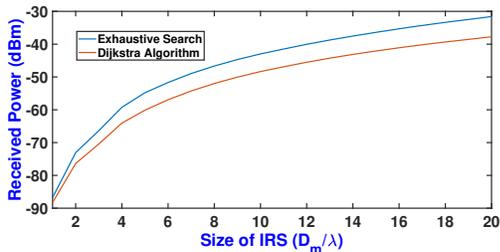
Fig. 5: Received power as a function of size of the IRS.
