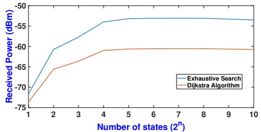
Fig. 7: Received power as a function of the number of states.
