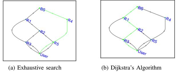
Fig. 4: Path selection using exhaustive search algorithm and dijkstra's algorithm
