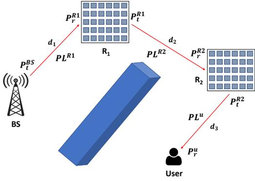
Fig. 2: IRS assisted path between the BS and the user.
