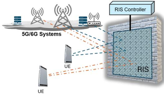
Fig. 1: A workflow of the RIS-assisted RAN concept
