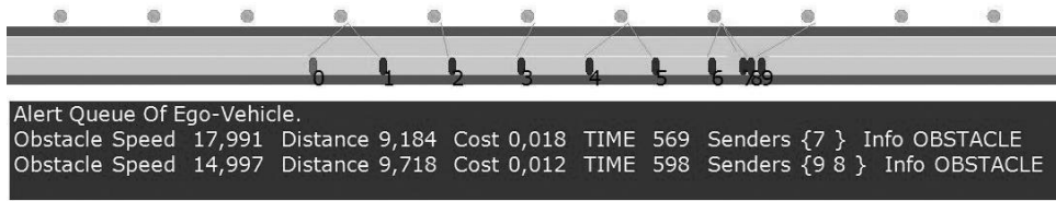
Figure 7.6: Ego-vehicle receives through the road infrastructure messages reported by i-vehicles with id numbers 7, 8 and 9.
