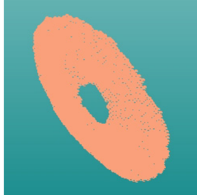
Figure 5.7 A feature representing the bottom of the screwdriver handle
