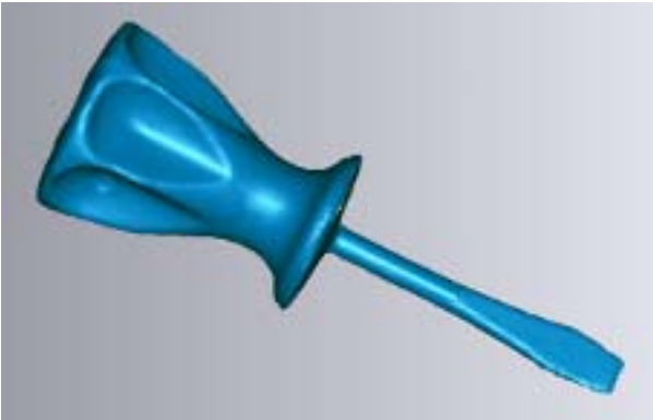
Fig. 19 Reconstructed B-rep model of the screwdriver.
