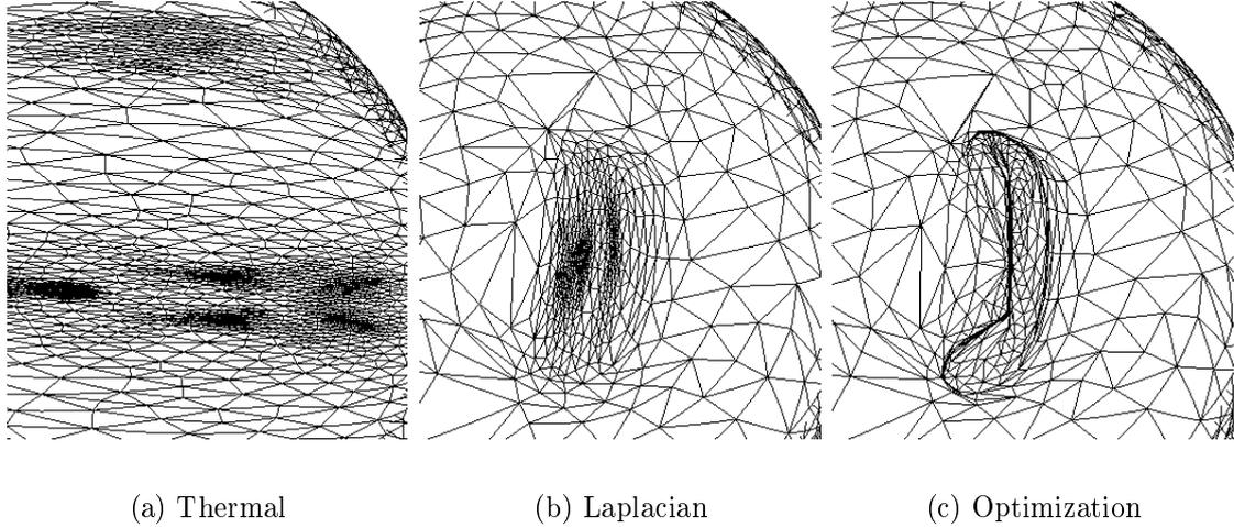
Figure 2.4: Close-up of the mapping from the monkey model. In the thermal mapping, although the mapping is valid it deviates from the original projection. The Laplacian mapping contains good quality triangles resulting from the smoothing process but loses some locality. Finally, the optimization balances between good quality triangles and preserving the mapping close to the original projected mapping. Note how the mapping is naturally distorted in concave areas around the ear.
