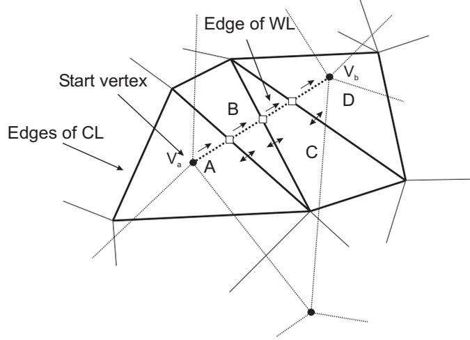
Figure 2.9: Calculating the Intersections of an Edge. Light edges are from  $M_a$ , Dark edges are from  $M_b$  Bold edges are those inserted in the Candidate List ( $CL$ ).
