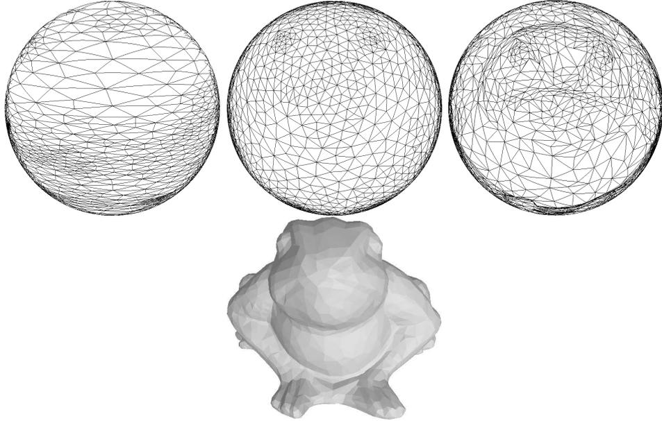
Figure 2.2: (top left) The result of initial mapping with the thermal conduction method, (top center) the result of the initial mapping with the Laplacian smoothing technique, (top right) the result of the mapping after optimization and (bottom) the original frog model.
