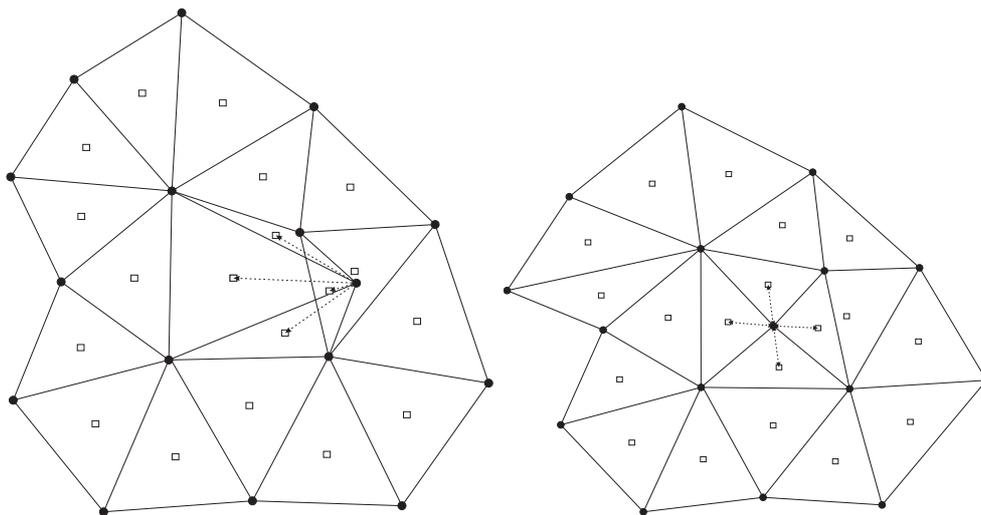
Figure 2.5: Geometric explanation of why Laplacian smoothing works. The original mesh (left) contains a node with folded elements, all the adjacent elements will act forces on that node forcing it to move in a balanced position (right). Consequently, all the folded elements will unfold after a certain number of iterations.
