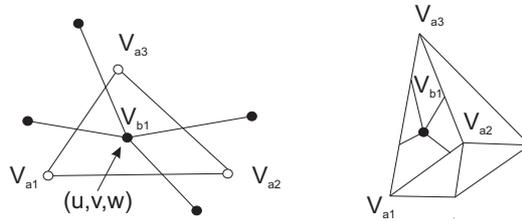
Figure 2.10: Mapping vertex  $V_{b1}$  of the second model to a face of the first model ( $V_{a1}, V_{a2}, V_{a3}$ )
