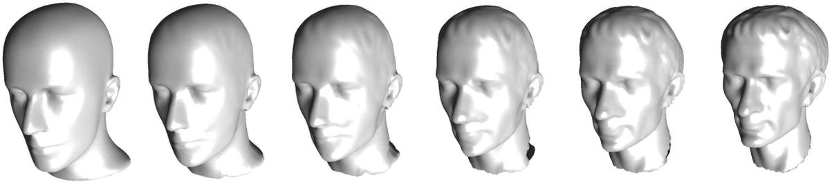
Figure 5.8: Morphing with alignment, merged topology has 127161 faces.
