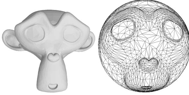
Figure 2.7: The final result of mapping (right) applied to the monkey with 5600 faces (left).
