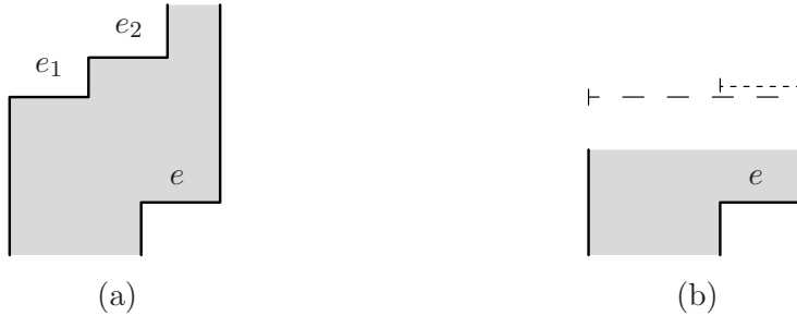
Figure 3: (a) A guard needs to be placed no higher than the N-edge e_2 to watch the S-edge e ; (b) the f-range (shown dotted) and the p-range (shown dashed) of the S-edge e .
