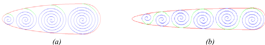
Figure 16. (a) Teardrop with four spirals. (b) Teardrop with three pairs of connected spirals.
