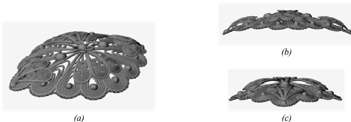
Figure 37. (a) The 3D CAD model of the brooch after bending is performed in two directions, (b),(c) side views of the brooch model after bending in the second direction.
