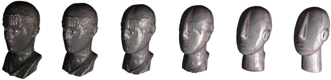
Figure 4.12: Morphing with alignment but no feature point matching of the Charioteer model (11098 faces) to a Cycladic idol model (16798 faces), merged topology has 142422 faces.
