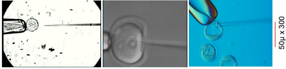
Figure 1.10: Cell injection using manipulator [1]
