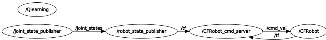
Figure 3.10: Navigation of centrifugal-force robot with Q-Learning nodes
