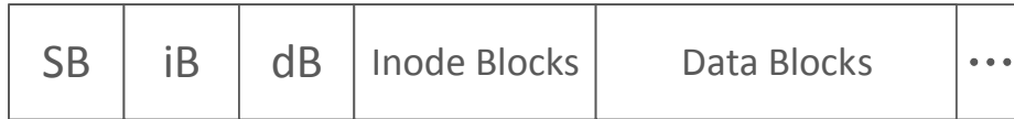
Figure 2.8: Organization of a novel file system: Superblock, Inode bitmap, Data block bitmap, Inode blocks and Data blocks
