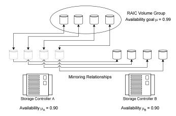
**Figure 10** Strengthening availability by mirroring across storage RAID array controllers. In this example, the two storage controllers are equivalent and characterized by availability  $\mu$ . Note that RAIC provides the failover capability required in case of failure of RAID controller A.
