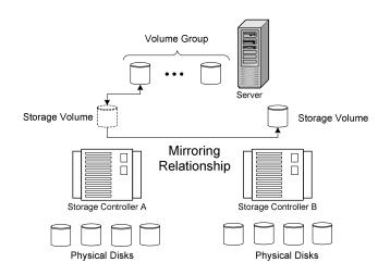
Figure 4 Volume mirroring is a data-redundancy mechanism provided at the front-end of RAID storage controllers on top of the redundancy mechanism (parity, block mirroring) that the RAID controller implements in its storage back-end. The higher-level mirroring policies (e.g., failover handling, etc.) must be specified externally by the agent that configures the mirroring relationship.
