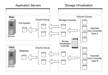
Figure 2 In this example, a storage virtualization controller imports storage volumes from storage controllers of type A and B into separate volume groups. Each storage volume exported by the virtualization controller is carved out of one of these volume groups. Note that this is equivalent to performing storage allocation using the one-to-one model.
