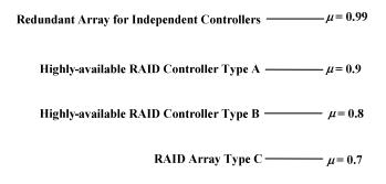
**Figure 7** A storage controller can dynamically move between availability levels based on its history and current confidence on its operating parameters. Achieving arbitrarily high levels of availability (such as  $\mu = 0.99$ ) may only be possible with techniques such as those used by RAIC.
