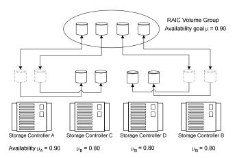
**Figure 11** Maintaining availability goals for a RAIC volume group as the latter grows and incorporates storage volumes across RAID controllers of varying capabilities. In this example, primary RAID controllers A and B are characterized by availability levels  $\mu_A$  and  $\mu_B$ , respectively. Secondary RAID controllers C and D are characterized by availability levels  $\mu_C$  and  $\mu_D$ , respectively.
