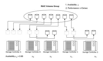
Figure 9 A realization of the VG configuration of Figure 8.
