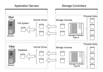
Figure 1 Storage volumes that make up a data object (e.g., a file system or a database table-space), map to a single storage controller in the one-to-one storage allocation model.
