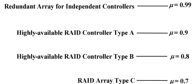
**Figure 7** A storage controller can dynamically move between availability levels based on its history and current confidence on its operating parameters. Achieving arbitrarily high levels of availability (such as  $\mu = 0.99$ ) may only be possible with techniques such as those used by RAIC.
