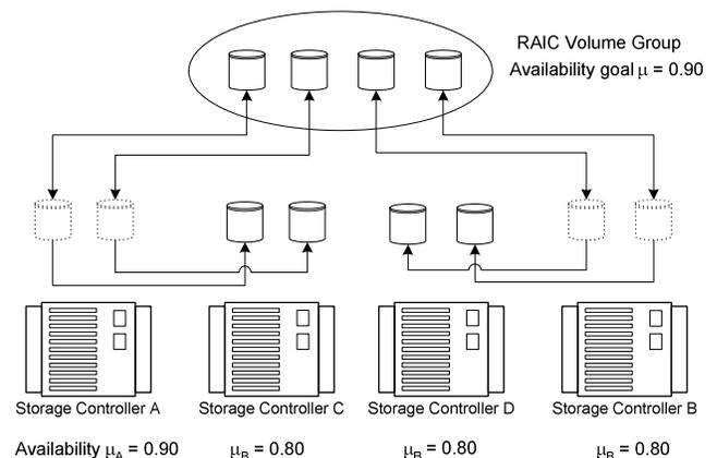
**Figure 11** Maintaining availability goals for a RAIC volume group as the latter grows and incorporates storage volumes across RAID controllers of varying capabilities. In this example, primary RAID controllers A and B are characterized by availability levels  $\mu_A$  and  $\mu_B$ , respectively. Secondary RAID controllers C and D are characterized by availability levels  $\mu_C$  and  $\mu_D$ , respectively.
