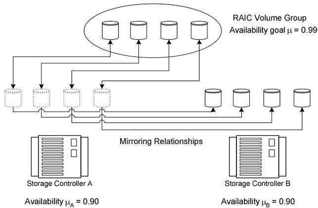
**Figure 10** Strengthening availability by mirroring across storage RAID array controllers. In this example, the two storage controllers are equivalent and characterized by availability  $\mu$ . Note that RAIC provides the failover capability required in case of failure of RAID controller A.
