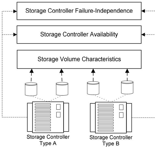
**Figure 6** Information about storage controllers and storage volumes collected and maintained by RAIC.
