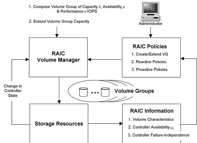
**Figure 5** The RAIC VM composes or extends VGs according to capacity, performance, and availability goals. RAIC responds to changes in controller-availability state using availability and performance classification of RAID controllers as well as administrator input.
