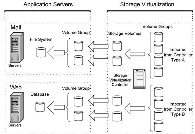
**Figure 2** In this example, a storage virtualization controller imports storage volumes from storage controllers of type A and B into separate volume groups. Each storage volume exported by the virtualization controller is carved out of one of these volume groups. Note that this is equivalent to performing storage allocation using the one-to-one model.
