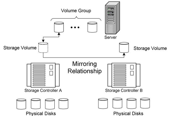
**Figure 4** Volume mirroring is a data-redundancy mechanism provided at the front-end of RAID storage controllers on top of the redundancy mechanism (parity, block mirroring) that the RAID controller implements in its storage back-end. The higher-level mirroring policies (e.g., failover handling, etc.) must be specified externally by the agent that configures the mirroring relationship.
