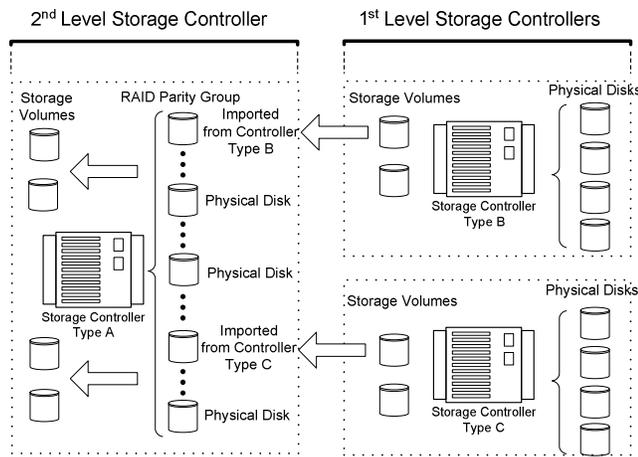
**Figure 3** In a multi-layered RAID scheme, higher-level RAID controllers can create RAID disk (or parity) groups from heterogeneous storage devices, which may include direct-attached physical disk drives as well as storage volumes imported from lower-level RAID controllers.
