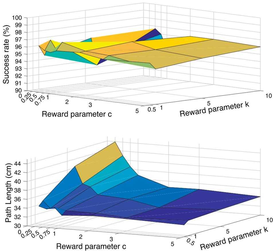
**Figure 7.** Evaluation of the impact of the reward function parameters  $k$  and  $c$  (Equations (11)) on the scenario (f). The diagrams show the *mean percentage of the successful episodes* and the *mean path length* taken from 1000 episodes of 20 learned policies obtained after executing 20 independent simulations. All simulation runs were made using the Single Q-learning scheme in the last scenario (f) that constitutes the most difficult case.
