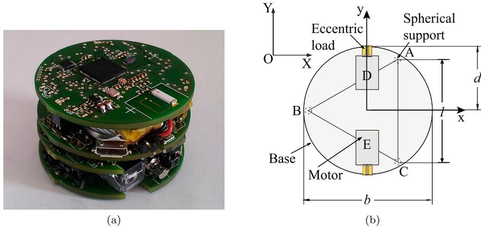
Figure 2. (a) Prototype; (b) Design concept (top view) (figures from [33]).
