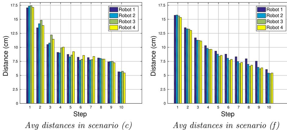
**Figure 11.** Average distances between each robot and their nearest neighbour during their trajectories (divided into 10 bins). The bars are obtained after executing 20 independent simulated runs in scenarios (c) and (f).
