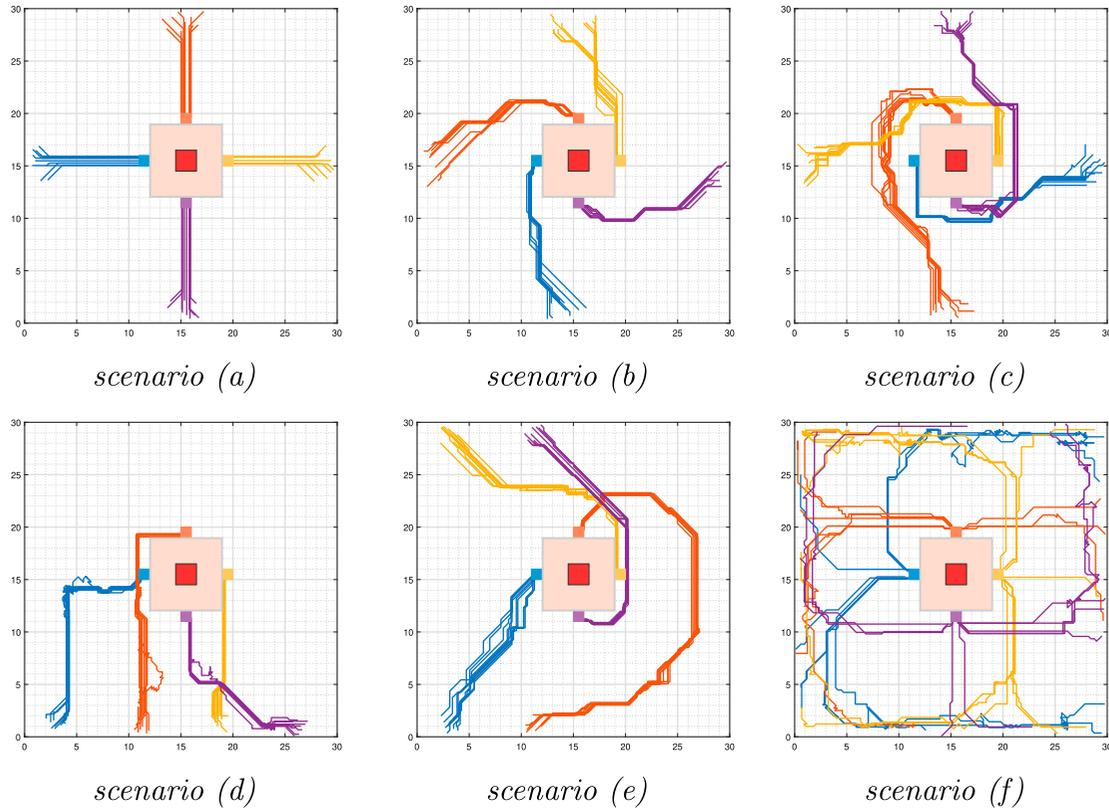
**Figure 10.** Exemplar trajectories for four mini-robots as obtained from the learned policies of the proposed multiagent RL approach using the Double Q-learning algorithm.
