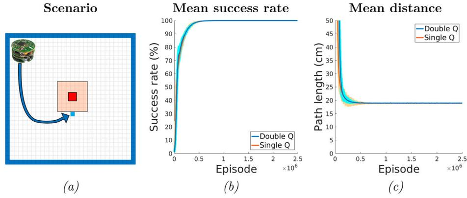
**Figure 5.** The simulated scenario used and the obtained comparative learning curves of the single mini-robot training. The curves represent the mean success rate and the mean path length needed to reach the target of double and single Q-learning algorithms, together with the standard deviation.
