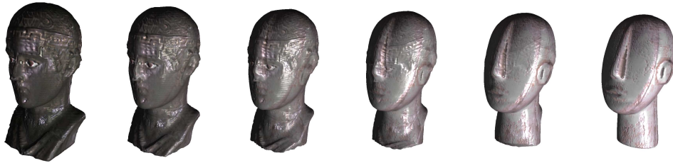
Figure 15: Morphing with alignment but no feature point matching of the Charioteer model (11098 faces) to a Cycladic idol model (16798 faces), merged topology has 142422 faces.
